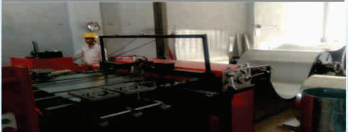
Auto Duct Forming Line FS 1500
